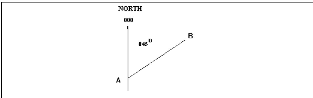
Measuring bearings in degrees [A - B = 045 degrees]
