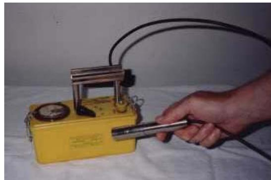
window is open it detects both beta and gamma. This survey meter is calibrated only for gamma radiation, so you can not get an accurate reading of the exposure rate from beta particles, only an indication of their presence.
