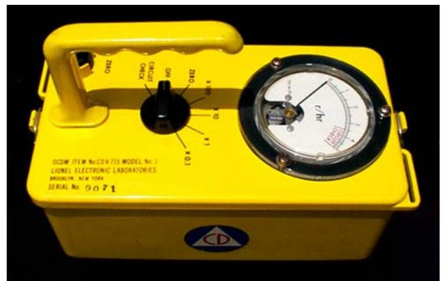
**CD V-717 Civil Defense High-Range Survey Meter** 0-500 R/hr range - 5.25 pounds, 3-part die cast aluminum case, watertight, will float. Powered with one D-sized battery, continuously for 150 hours, longer if on intermittent basis.
