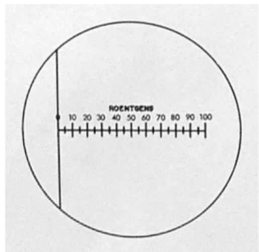
It's also similar to the odometer of a car; where both measure an accumulation of units. The dosimeter will indicate a certain total number of R or mR exposure received, just as the car odometer will register a certain number of miles travelled.
