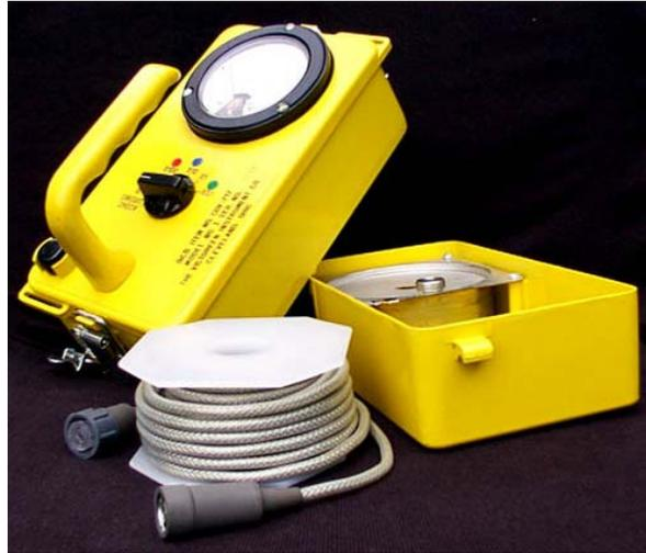
**CD V-720 Civil Defense High-Range Survey Meter** 0-500 R/hr range - 3.75 pounds, 2-part die cast aluminum case, watertight, will float. Powered with two D-sized batteries, continuously for 150 hours, longer if on intermittent basis.
